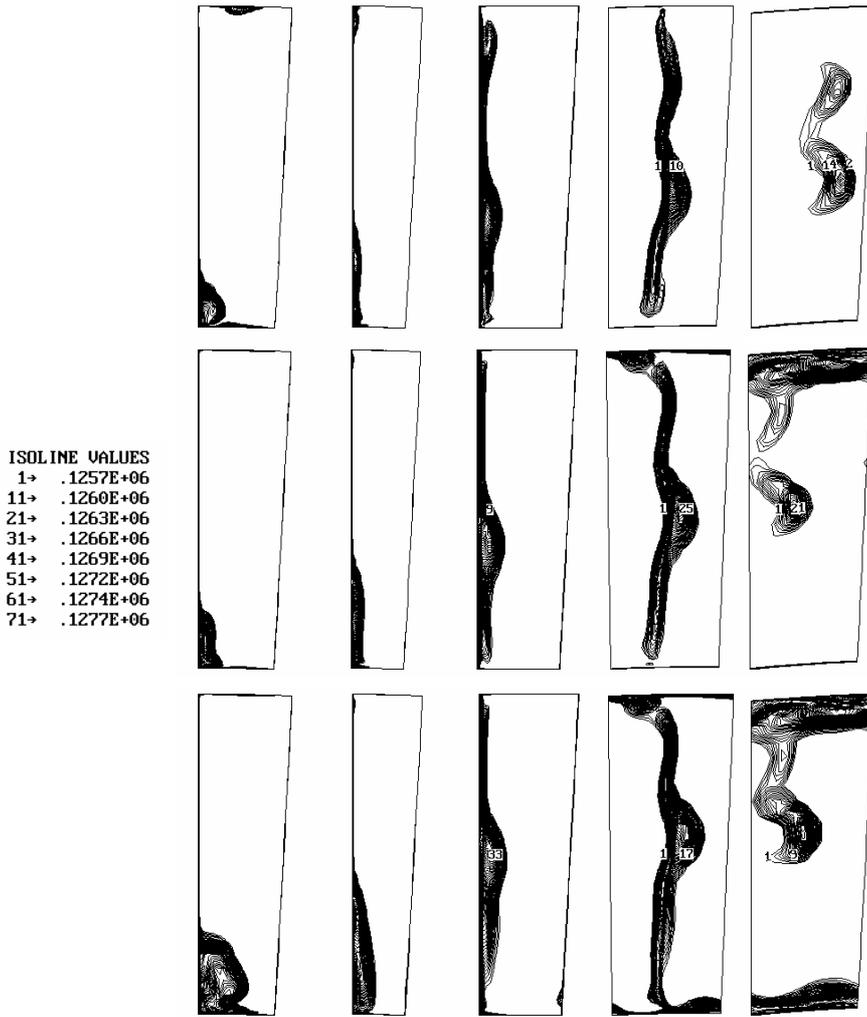
Fig. 5. Entropy function contours in the rotor at 10%, 52%, 96% axial chord from the leading edge, and downstream of the rotor at 10% and 45% axial chord from the trailing edge - computed without sources and sinks (top), computed with tip leakage (centre), computed with tip leakage and windage flows (bottom).
