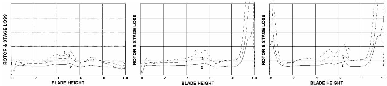
Fig. 8. Span-wise distribution of kinetic energy losses in the rotor (1), stage without the exit velocity (2) and with the exit velocity (3) -computed without sources and sinks (left), computed with tip leakage (centre), computed with tip leakage and windage flows (right).
