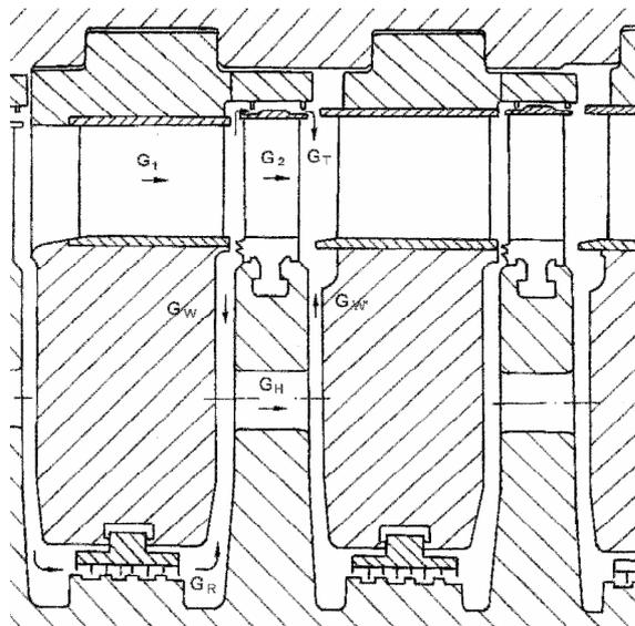
Fig. 1. Impulse turbine geometry.
