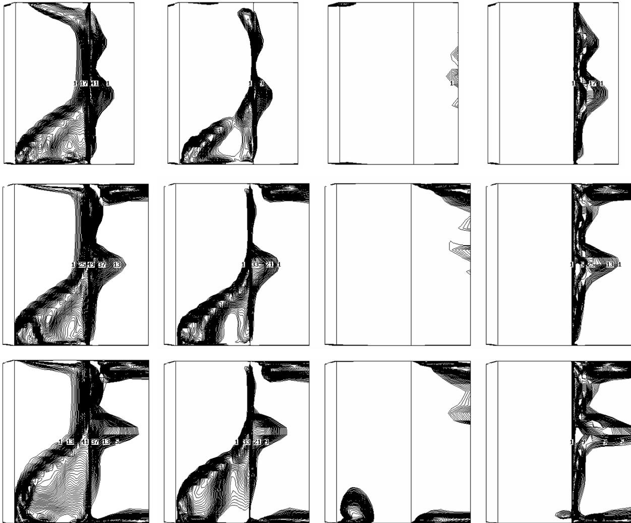
Fig. 4. Entropy function contours in meridional view in the computational domain of the rotor at 3% (left), 12% (centre left), 48% (centre right) and 96% (right) blade-to-blade distance from the suction surface - computed without sources and sinks (top), computed with tip leakage (centre), computed with tip leakage and windage flows (bottom).
