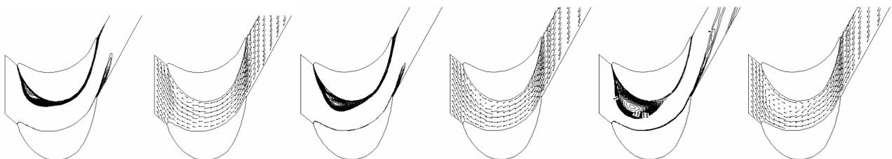
Fig. 7. Entropy function contours and velocity vectors in the rotor at 9% blade span from the root - computed without sources and sinks (left), computed with tip leakage (centre), computed with tip leakage and windage flows (right).
