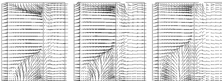
Fig. 6. Velocity vectors in the rotor at the suction surface - computed without sources and sinks (left), computed with tip leakage (centre), computed with tip leakage and windage flows (right).
