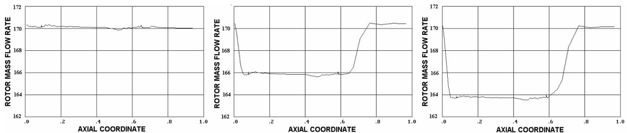
Fig. 3. Axial distribution of mass flow rate in the computational domain of the rotor - computed without sources and sinks (left), computed with tip leakage (centre), computed with tip leakage and windage flows (right).
