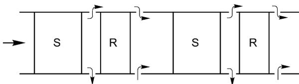
Fig. 2. Computational domain with source/sink-type permeable boundaries to simulate the effect of leakage over shrouded rotor blade tips and windage flows; S - stator, R - rotor.
