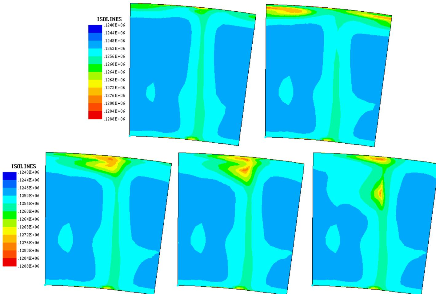
Fig. 8. Entropy function contours in the normal plane downstream of the second stator: tip leakage jet flow rate 1% and 3%; swirl angle  $0^\circ$ , meridional angle  $-90^\circ$  (top); tip leakage jet flow rate 3%; swirl angle  $40^\circ$ ,  $60^\circ$  and  $80^\circ$ , meridional angle  $-90^\circ$  (bottom).
