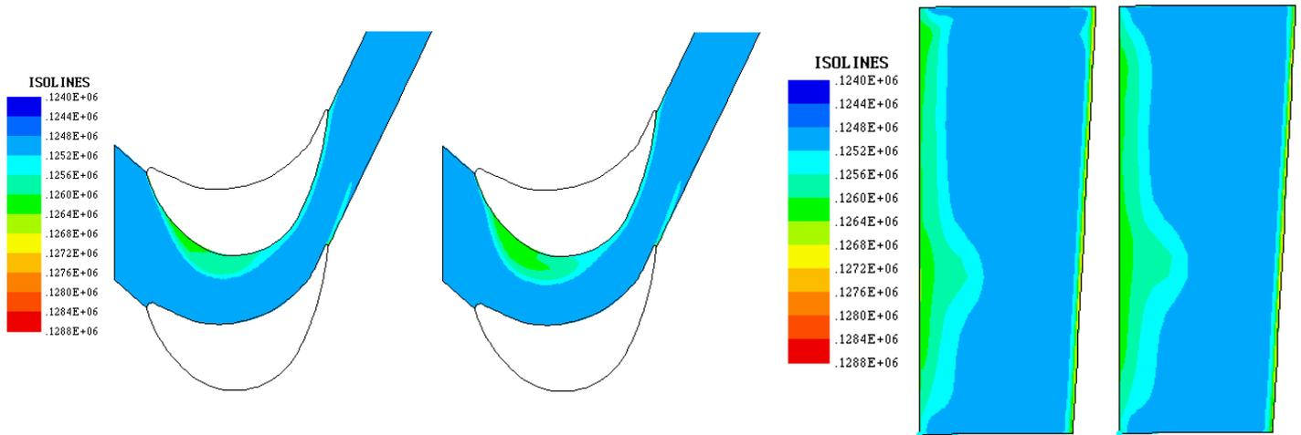
Fig. 5. Entropy function contours in the blade-to-blade plane of the first rotor 10% blade height from the hub (left) and in the normal plane at the rotor trailing edge (right) for leakage mass flow rate 1% (left) and 3% (right).
