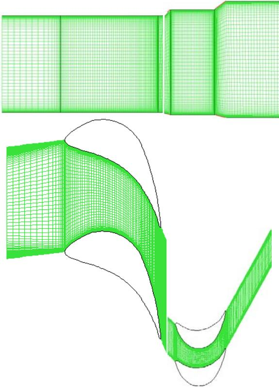
Fig. 3. Model air turbine – computational grids for the stator and rotor cascades in meridional view (top), and blade-to-blade section (bottom).
