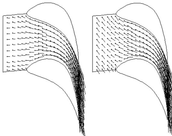
Fig. 7. Velocity vectors in the second stator 8% blade height from the tip for the tip leakage jet swirl angle  $0^\circ$  (left) and  $80^\circ$  (right); leakage flow rate 3%, meridional angle  $-90^\circ$ .
