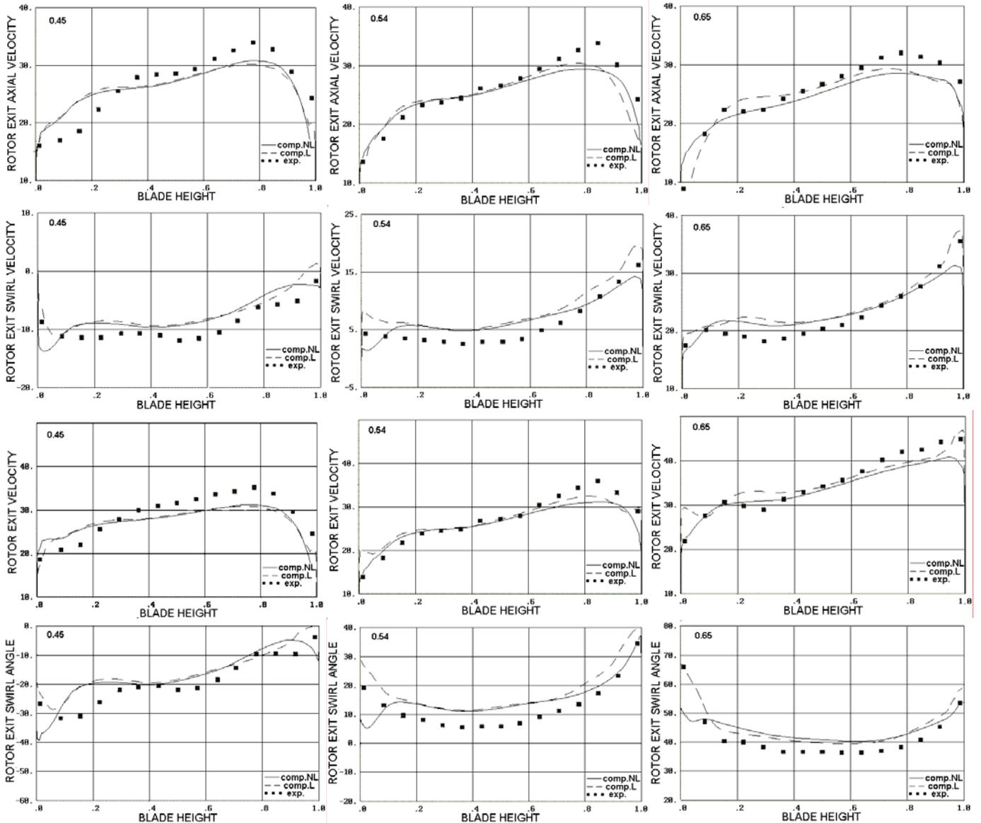
Fig. 4. Model air turbine - computed and experimental axial velocity (top), absolute swirl velocity (top centre), absolute velocity (bottom centre) and absolute swirl angle (bottom) at the rotor exit:  $u/c_{0T}=0.45$  (left), 0.54 (centre), 0.65 (right); comp.NL – computed without leakages, comp.L – computed with root and tip leakages, exp. – experimental.
