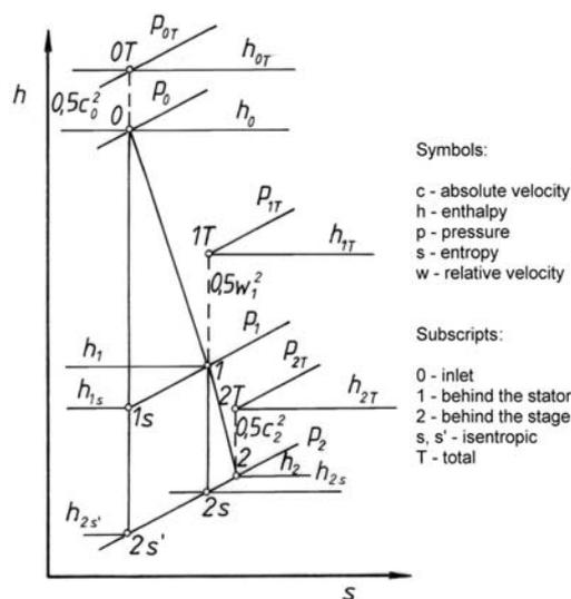
Fig. 10. Enthalpy-entropy diagram for a turbine stage
