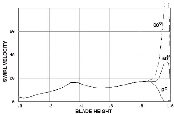
Fig. 6. Absolute swirl velocity at the rotor exit for three values of tip leakage jet swirl angle  $0^\circ$ ,  $50^\circ$  and  $80^\circ$ ; leakage flow rate 3%, meridional angle  $-90^\circ$ .
