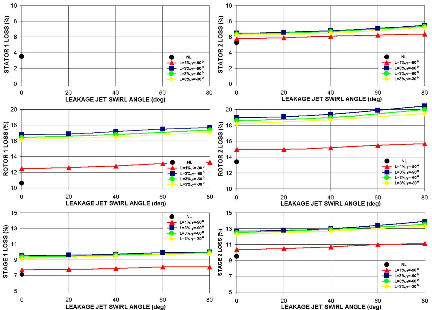
Fig. 9. Mass averaged enthalpy losses in the first stator, rotor and stage (left), second stator, rotor and stage (right) as a function of tip leakage jet swirl angle at re-entry for two leakage flow rates of 1% or 3% and three leakage jet meridional angles  $-90^\circ$ ,  $-60^\circ$ ,  $-30^\circ$ . Computational results without leakage are indicated by a black circle. Enthalpy losses in the first stator do not change when the leakage is modelled.
