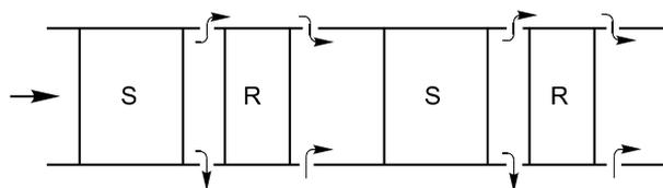
Fig. 2. Computational domain with source/sink-type boundaries; S - stator, R - rotor.
