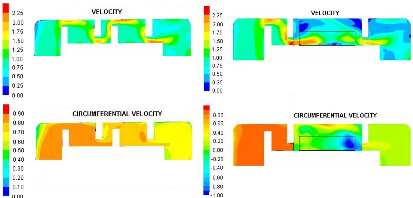
Fig. 1. Velocity magnitude and circumferential component of the velocity for a classical labyrinth seal (left) and a labyrinth seal with shroud bladelets (right)\*.
