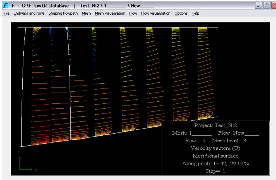
Fig. 4. Velocity vectors in meridional section of last row of 2½ stage compressor (postprocessor of F software package)
