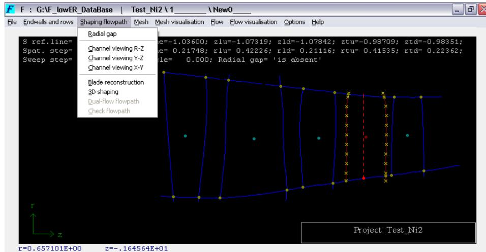
Fig. 2. Flowpath of 2½ stage compressor (preprocessor of F software package)
