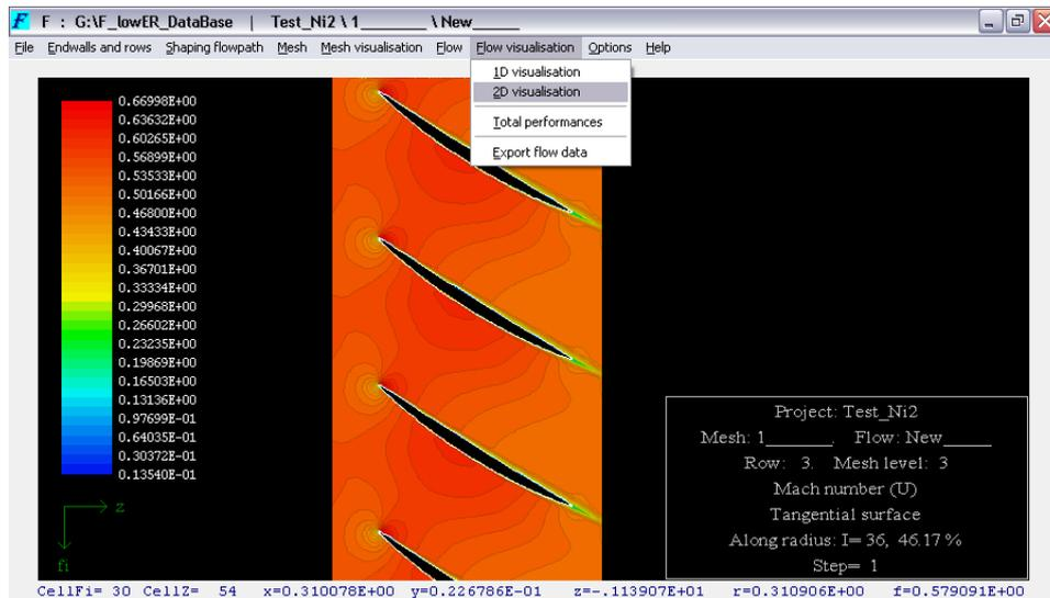
Fig. 3. Mach number contours in compressor cascade (postprocessor of F software package)
