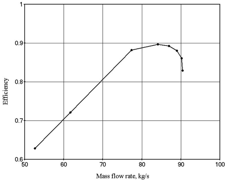
Fig. 6. Computed compressor performance
